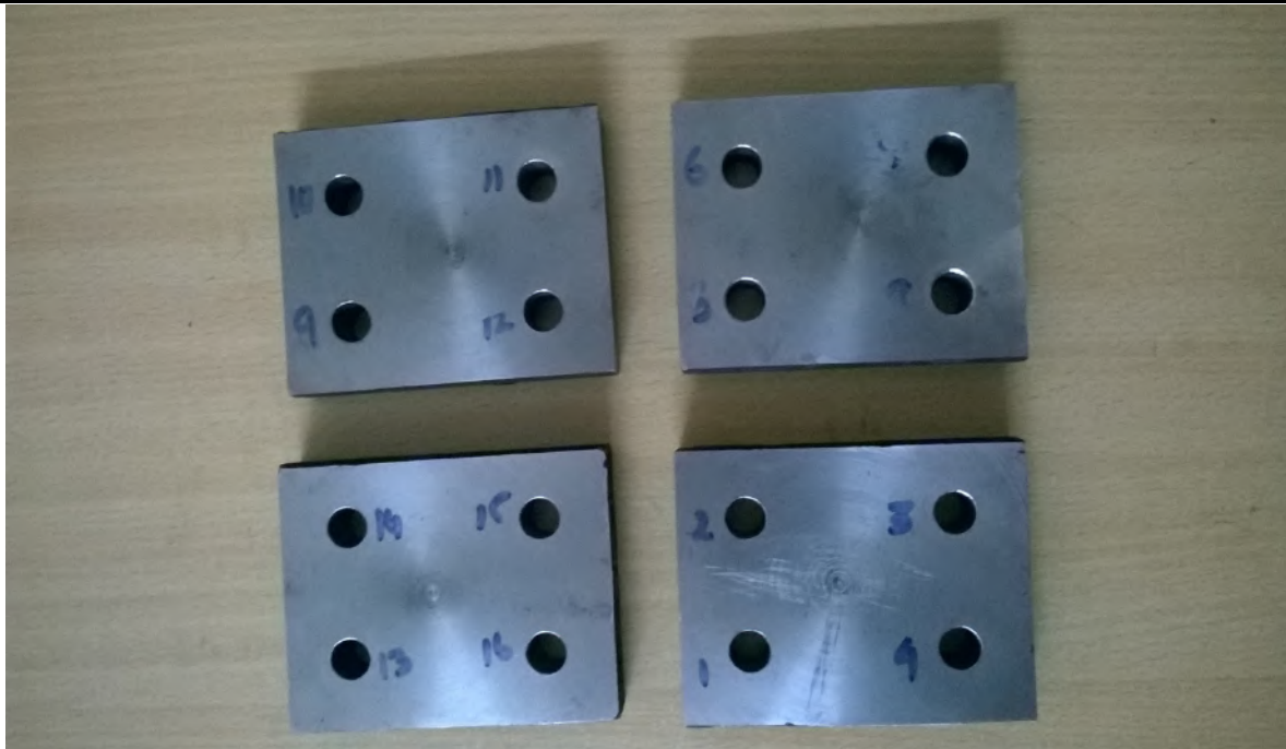
Fig.2: H13steel drilled specimen ( L_{16} )
